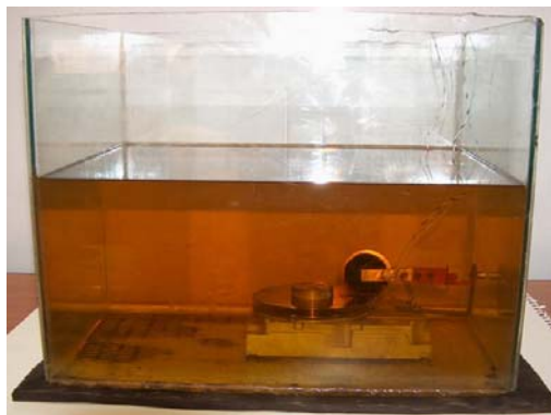
Figure 10. Unprotected submersible piezoelectric motor immersed in insulating oil.
