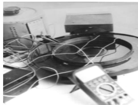
Figure 3. Experimental stand for the study of an electric motor with liquid rotor
