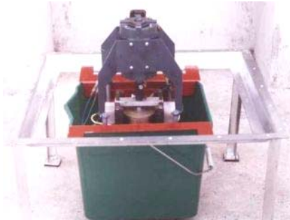
Figure 4. Experimental stand for the study of acyclic generator operating like an unprotected submersible electric machine (reproduced from: [9]).
